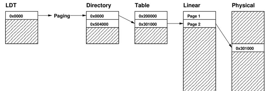
Our LDT descriptor 0x0000 points to a base address of 0x0. The paging mechanism translates this and passes us along to the Page Directory. Since we are operating within the first 4 megabytes of address space it forwards us to the first page table. The offset we supplied is the first byte in the second page, so the translation passes us along the chain through linear memory and on to our physical address of 0x301000. A few details were missed along the way, but that is basically what happens.
