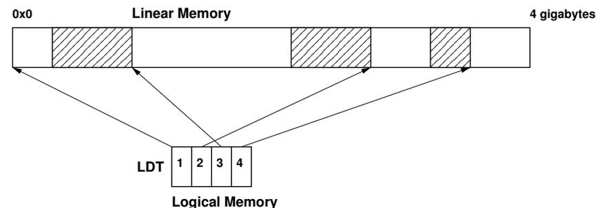
The empty boxes of linear memory represent arbitrarily sized segments. The LDT boxes are individual segment descriptors. The numbers inside the segment descriptors are called segment selectors. Specifying a logical address is the same as it was 20 years ago, except the offset could be just about anything. For example, if segment 1 had a size(or "limit") of 2 megabytes, the logical address 0x0001:00040558 is perfectly legitimate.
