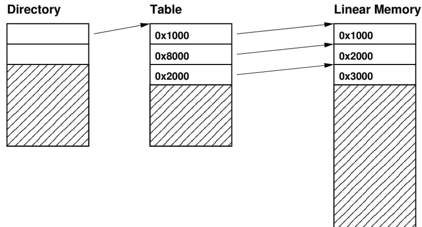
The addresses in the table entries are the physical base addresses of each page being pointed to, where the addresses listed in linear memory are what software will see. The maximum amount of memory we can address with a full Page Directory and full Page Tables under it totals 4 gigabytes, assuming we are using the default page size of 4k<sup>2</sup>.
