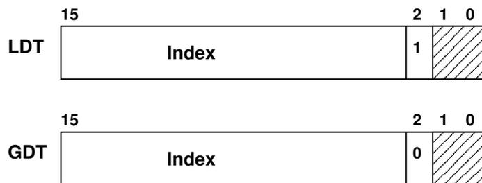
The grayed out areas in the selectors are a Requested Privilege Level field occupying 2 bits of space in the selector. The Index section is simply an index into the descriptor table containing the segment descriptor for the selector. The main difference between these two selectors is bit 2, the Table Indicator(TI) bit. When set, the selector is for a segment contained in the current Local Descriptor Table. When cleared, the selector indexes a segment in the GDT.
