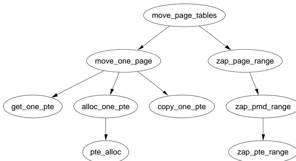
Figure 5.6: Call Graph: `move_page_tables()`**Function:** `move_page_tables` (*mm/mremap.c*)
